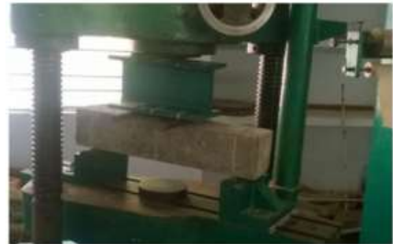
Testing Square prism for flexural strength
