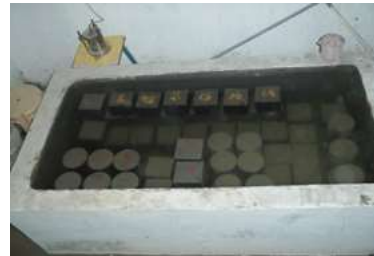
Curing of specimens for 7 days, 14 days and 28 days age
