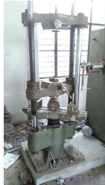
Split tensile strength testing at 14 days curing
